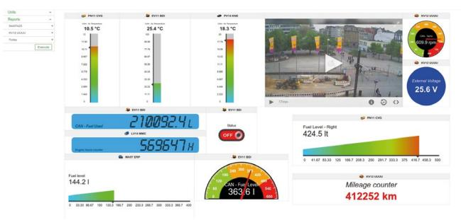
This tool comes in handy for controlling dozens of parameters of diesel generators, cooling and freezing chambers, and other stationary assets. The panel is used to visualize values of counters and sensors from any number of assets. Use it both for online monitoring and performance analysis based on historical data.
