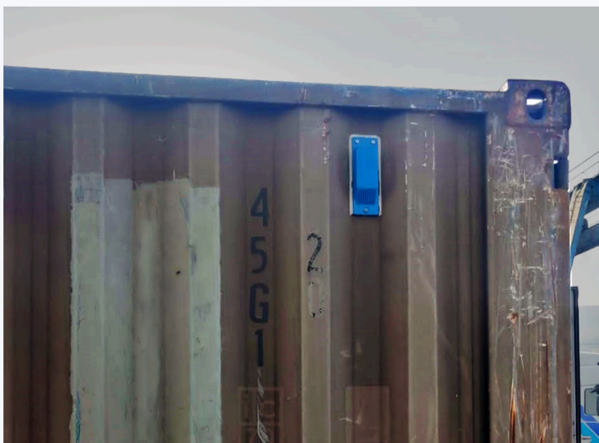
The housing with the telematics equipment inside, fixed on the wall of the freight container
