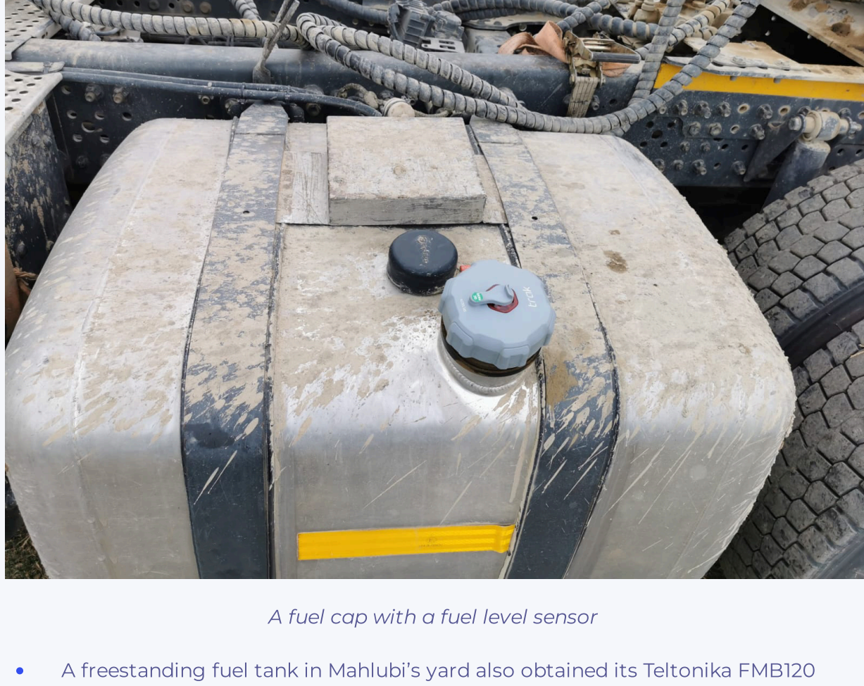
A fuel cap with a fuel level sensor
