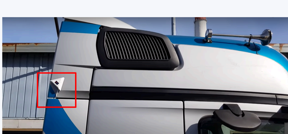
An infrared motion sensor on the cab looking over on the fuel tank. Fuel theft alarm is activated by this sensor
