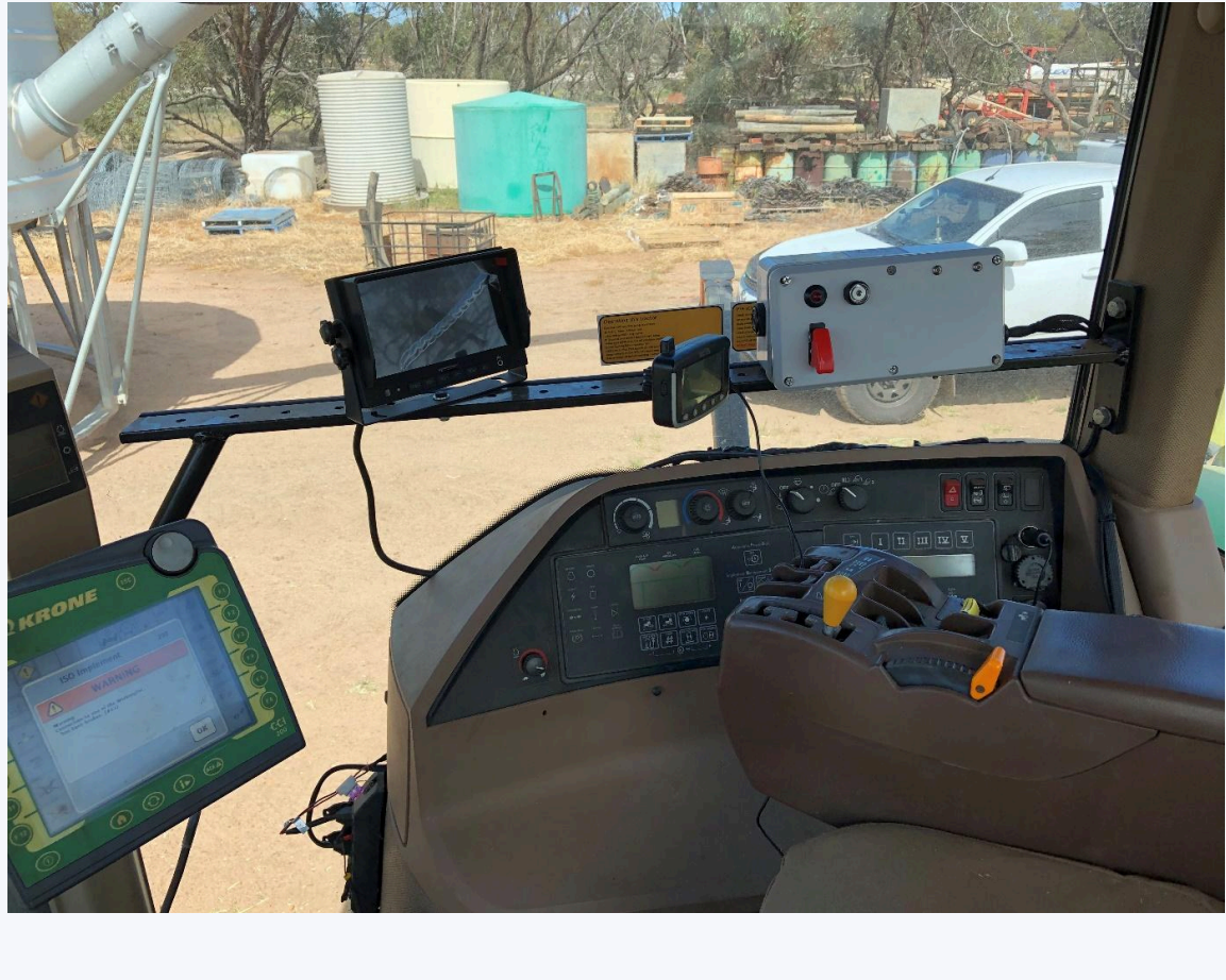
The white box with a tracking device, an iButton reader, and the button that a driver presses to record rebales
