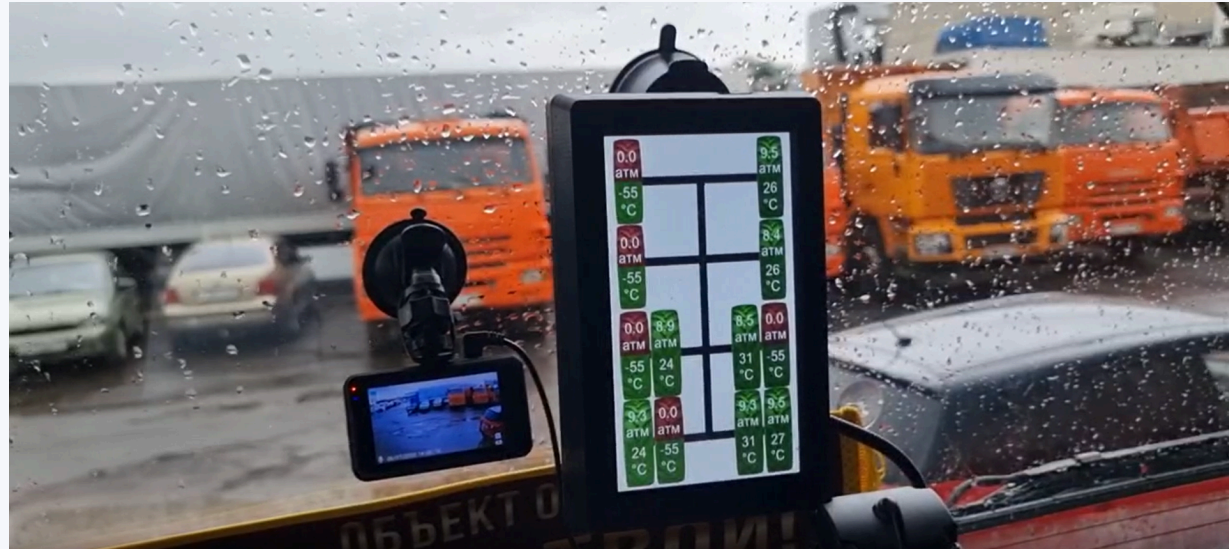
The display shows data on the condition of each wheel of the dump truck
