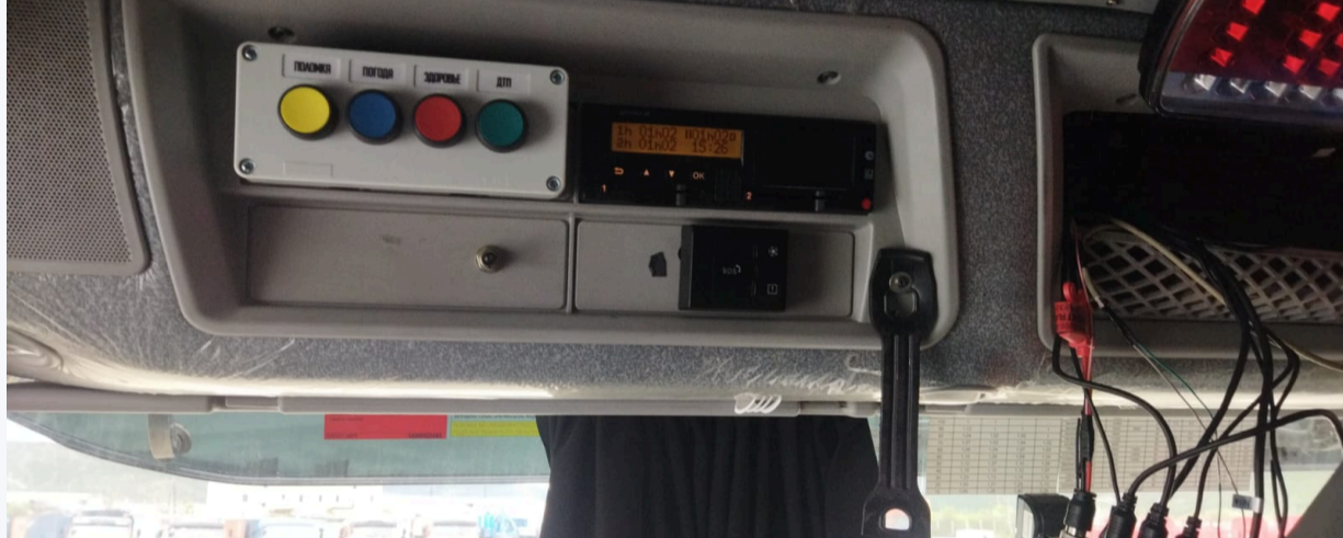
A four-button driver alert system mounted inside driver's cabin
