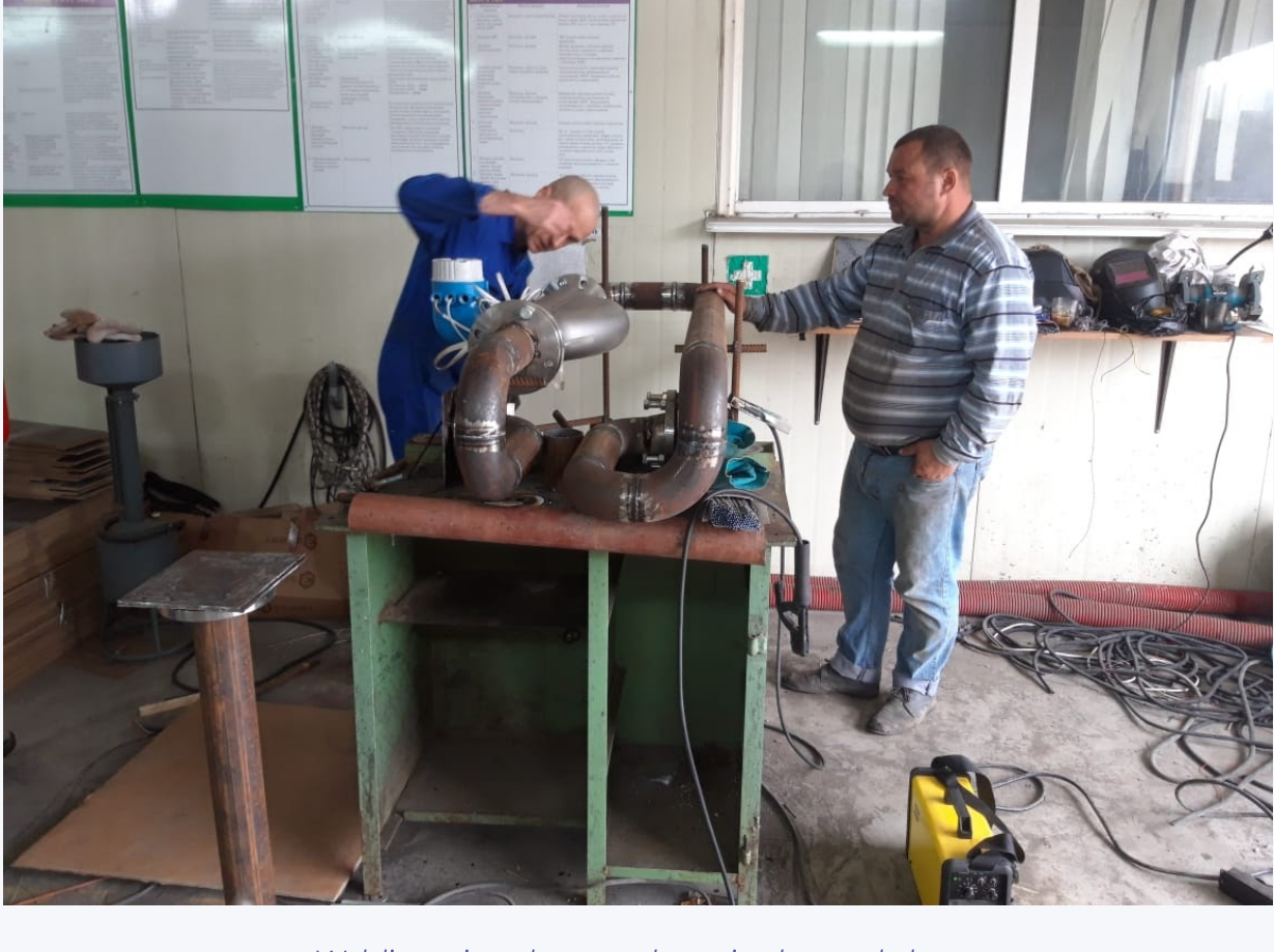
Welding pipes by templates in the workshop
