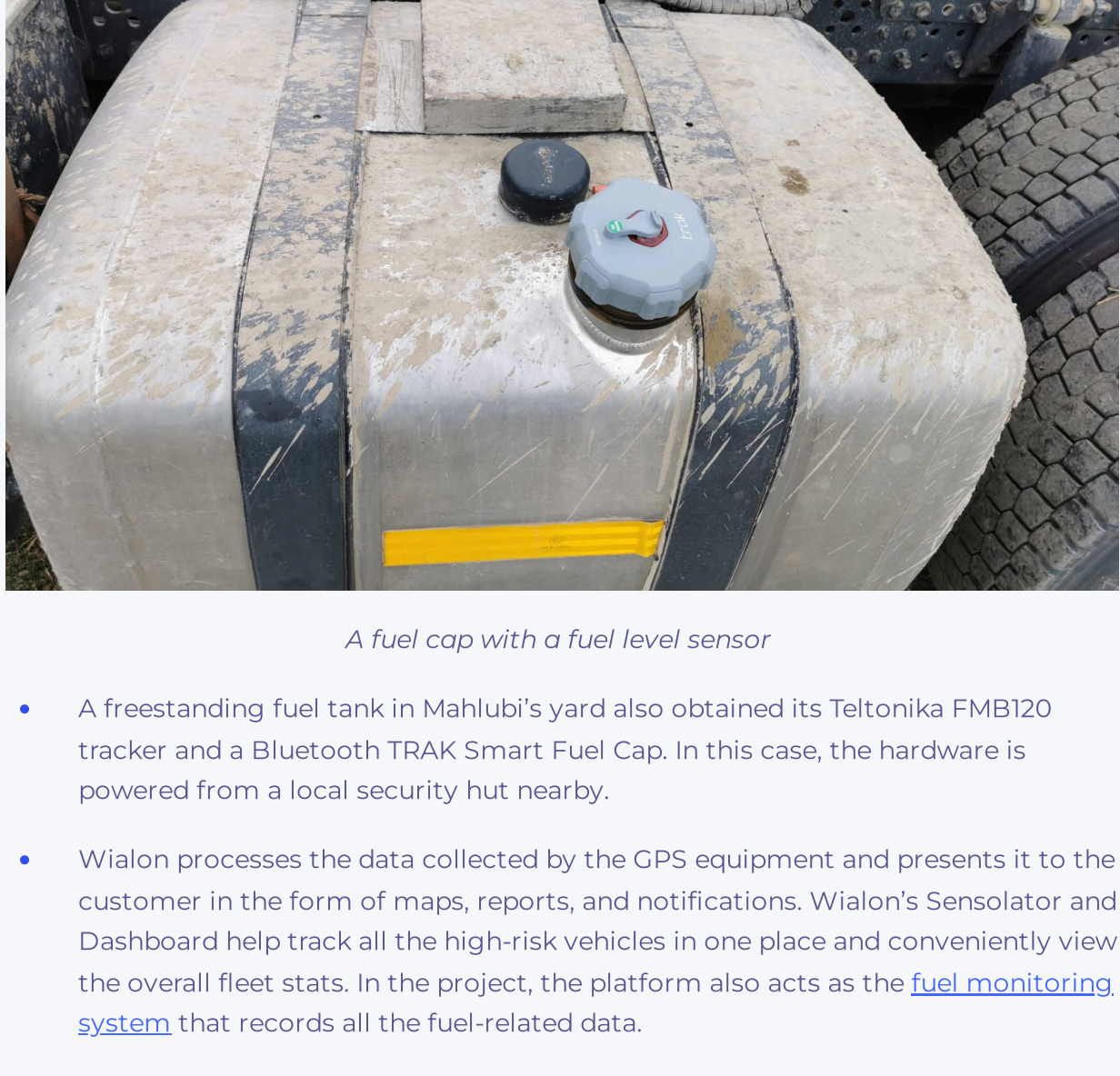
A fuel cap with a fuel level sensor
