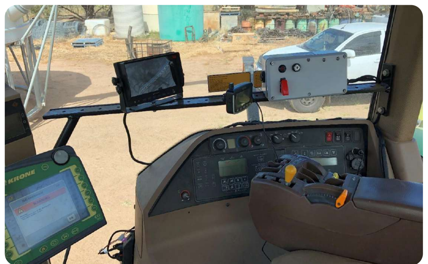
THE WHITE BOX WITH A TRACKING DEVICE, AN IBUTTON READER, AND THE BUTTON THAT A DRIVER PASSES TO RECORD REBALES
