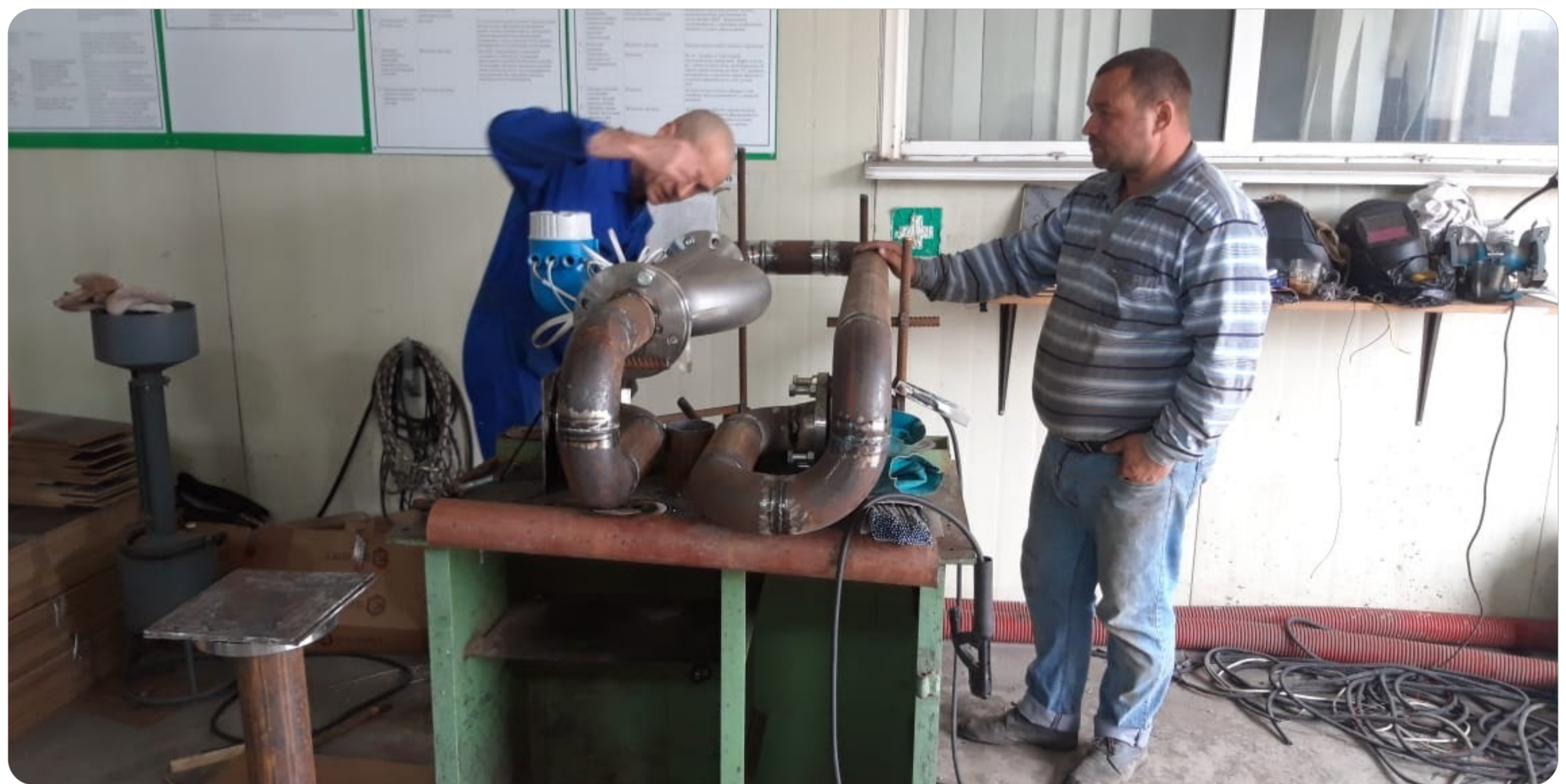
WELDING PIPES BY TEMPLATES IN THE WORKSHOP
